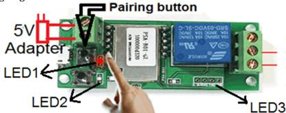
Connect these wires either to the wall switch terminals of the main unit opener or directly to the wall switch
