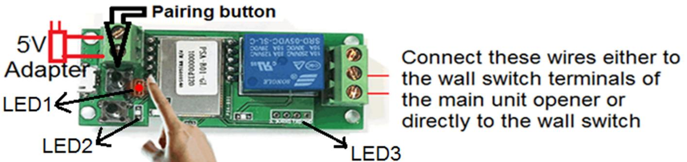
After installing the app and making sure that it works correctly (a clicking sound can be heard when you turns the switch On/Off by app or manually by pairing button) go to **wiring section** and connect your wifi device to your shutter door opener. Connect the 3 wires of this device either to the wall switch terminals of the main unit opener or directly to the wall switch wires. **After wiring you need to set up your inching mode time.**
