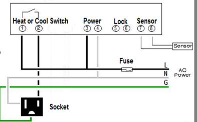
To prevent the frequent ON/OFF action of the output a temperature band (called hysteresis or differential set value) is created between the ON and OFF operations. The controller will use a range (a maximum and minimum) for process control action, which is between  $1^{\circ}$ C to  $15^{\circ}$ C. For example when the hysteresis is set on 5 and the set point on  $50^{\circ}$ C, the output ON/OFF action would be when the temperature goes lower than  $45^{\circ}$ C and higher than  $55^{\circ}$ C.
