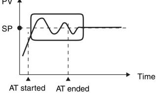
When it need artificially exit during **Auto-tuning**, set the Parameter(AT) to 0 so that can exit, but the setting result will not be valid.
