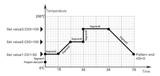
7.3 Parameter setting: Press SET+◀ enter into Program Setting Level
