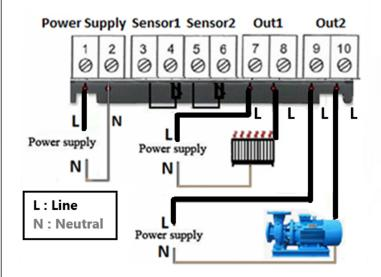
Out2 is for differential value (T2-T1) and Out1 is thermostat for T1(Lower temperature)
