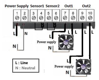
You can connect outputs like series and parallel for Special application too.
